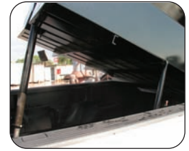
Inverted Front Mount Hoist, Rigid Body Understructure with Integrated Safety Body Prop
