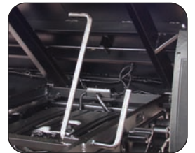
Sturdy Underbody with Integrated Safety Body Prop
