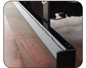
Fold Down Removable Sides with Dirt Shedding Lip
