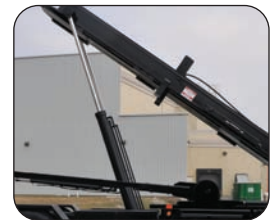
Forward Facing Tipping Cylinders for Better Lifting Efficiency
